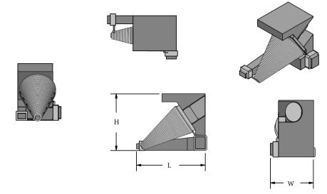
Note: Terminal is configured to facilitate attachment close to inductor tip. Wire is copper plated with gold 20  $\mu$  in.  $\pm 5 \mu$  in.
