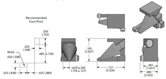
Note: Terminal is configured to facilitate attachment close to inductor tip. Wire is copper plated with gold 20  $\mu$  in.  $\pm 5~\mu$  in.
