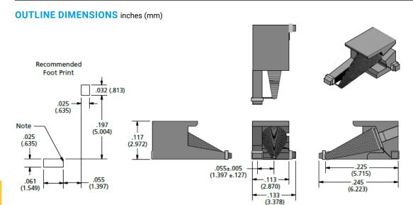
Note: Terminal is configured to facilitate attachment close to inductor tip. Wire is copper plated with gold 20  $\mu$  in.  $\pm 5~\mu$  in.
