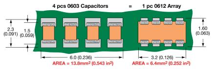
The 0612 4-element capacitor array gives a PCB space saving of over 50% vs four 0603 discretes and over 70% vs four 0805 discrete capacitors.
