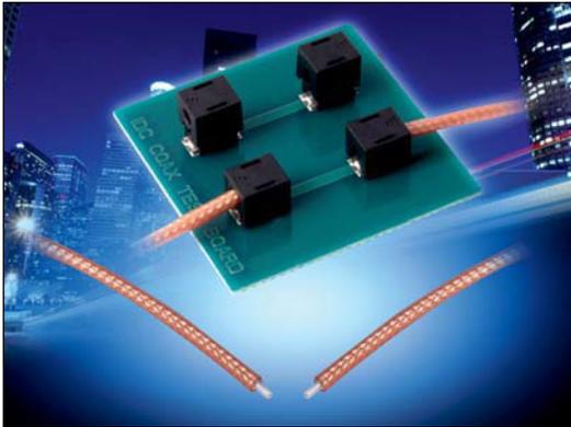
KYOCERA AVX has developed a unique 50 Ohm SMT Coax Connector based on our industry proven discrete wire Insulation Displacement Connector (IDC) technology. By combining two different sized IDC contacts, we can reliably pierce the center conductor and outside jacket dielectric materials to make electrical connection to the signal wire and braid (ground connection). Designed specifically for RG178 cable, the concept can be applied to other cable sizes.
