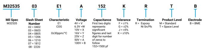
Packaging, Waffle as standard, for Tape and Reel add \1 to end of the part number, e.g. M3253503E1Z152KRTB\1 Please note all parts are terminated with a minimum 10% Pb plating.
