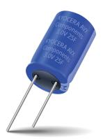
The new series of cylindrical electrochemical double-layer capacitors offers excellent pulse power handling characteristics based on the combination of very high capacitance and very low ESR. Used by themselves or in conjunction with primary or secondary batteries, they provide extended back up time, longer battery life, and provide instantaneous power pulses as needed. Offers great solutions to Hold Up, Energy Harvesting, and Pulse Power Applications.
