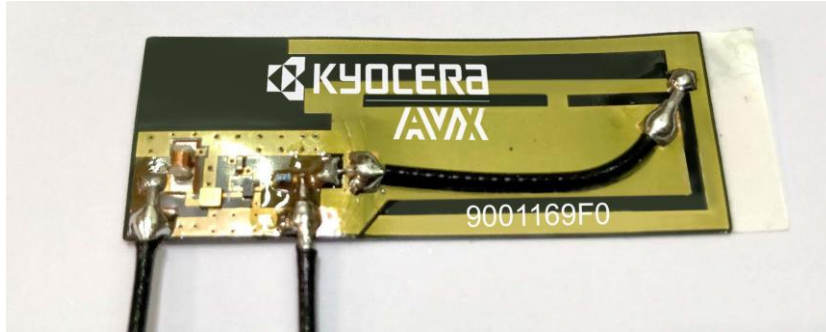
Additional 100mm u.fl cable is soldered to evaluate the active circuitry.
